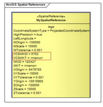
Looking at the WKT Tagged Value in the Tagged Values window for this element, you can see that the 'WGS 1984 Australian Centre for Remote Sensing Lambert Projected Coordinate' system has been selected.
